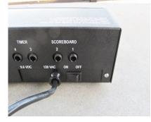
3. Turn the power on that goes to the scoreboard by pressing the ON switch located in the covered power box under the countertop next to the power plug outlet.
